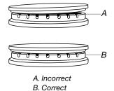
**5.** Turn on the burner. If the burner does not light, check cap alignment. If the burner still does not light, do not service the sealed burner yourself. Contact a trained repair specialist.
